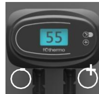
Pay attention to correct polarity when connecting!
