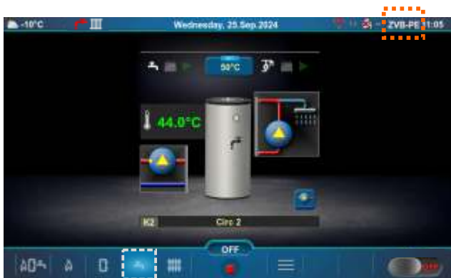
Domestic hot water (DHW) tank screen (ZVB-SE)
